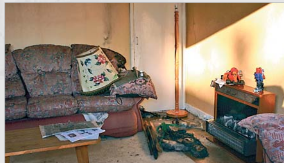
Furniture inside a flat WITH domestic sprinkler protection after combustion.
